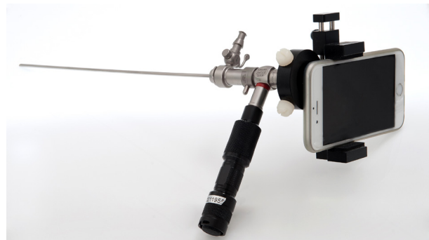
Figure 1: Portable hysteroscopic setup. The rigid hysteroscope coupled with iPhone 6s and portable LED light source
